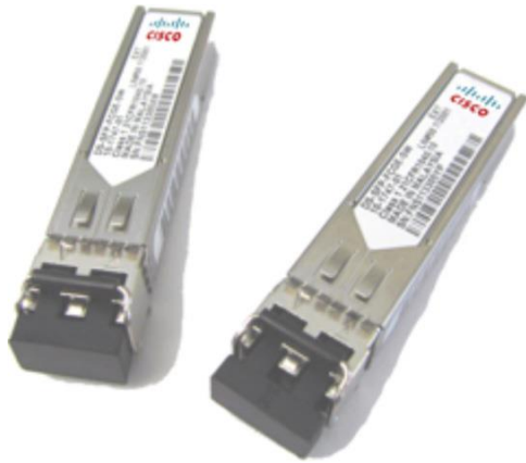
Figure 2. Cisco 4-Gbps Fibre Channel SFPs
